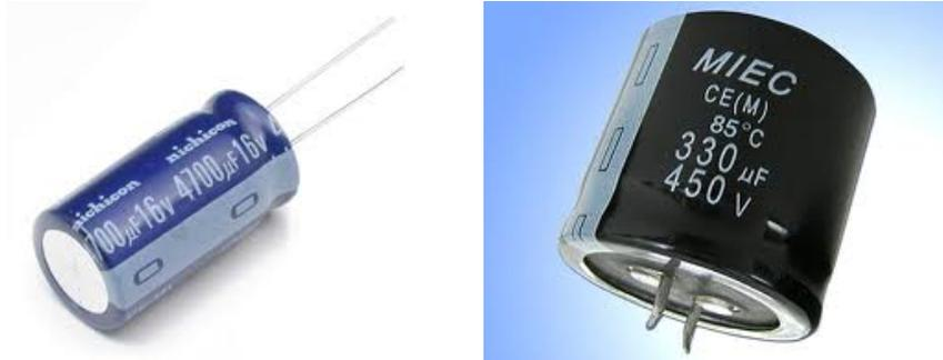
Also if the capacitor has wires, the minus wire is the shortest one!
