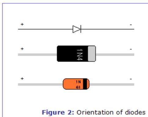
Figure 2: Orientation of diodes
