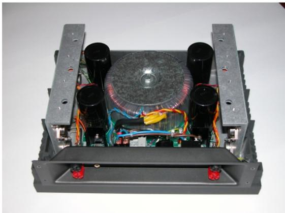
The unit will look like this. Remove the amplifier boards with a long Philips (posidriv no 2) screwdriver; be careful not to make contact with the components on the boards. Remove (loosen) the connectors on the boards with small pliers. Make notes about the position and the colors, or pictures.
