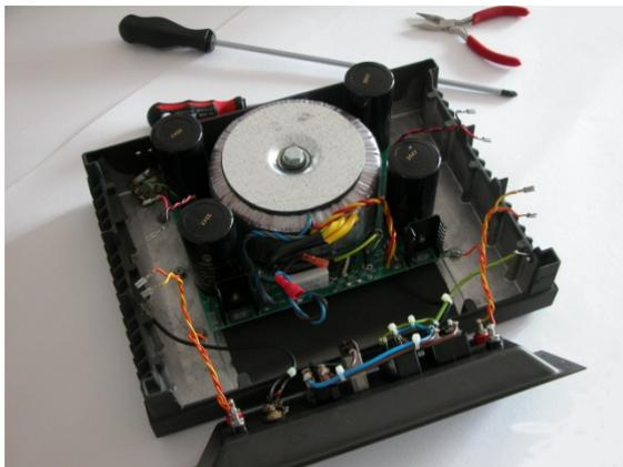
Remove the connectors from the PSU, make notes, or pictures! There is no need for soldering here. There are four large posidriv screws around the transformer, remove those. Be careful, sometimes they are a little bit covered by the transformer.
