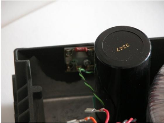
Remove the led circuit board from the front of the amplifier
