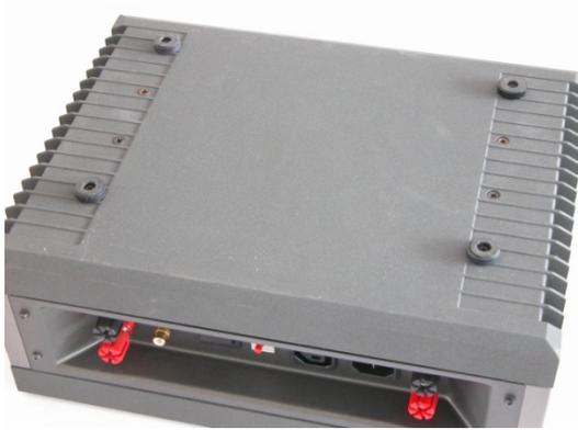
Remove the 8 screws on the bottom and the 4 screws from the rear panel. Remove the bottom and the U shaped chassis part.
