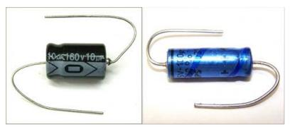
With axial capacitors there is an extra arrow indicating the minus wire, or there is a printed small ring around the body indicating the minus wire. Also the minus wire is direct connected to the aluminium body. The plus wire is sticking through the black plastic cap.
