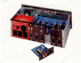
The Quad 44 preamp was the first Quad preamplifier using op-amps and electronic switches. The input circuits where built as separate modules, allowing for more versatility. The input modules are interchangeable, so you could equip the unit with 5 pickup inputs or any other combination.
