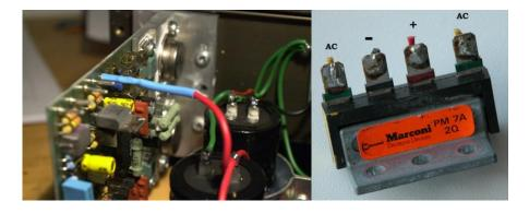
It is no luxury to use some Raychem (or other) Heat Shrinkable Tubing for insulating the +, - and output connections, as there are large voltages between them.
