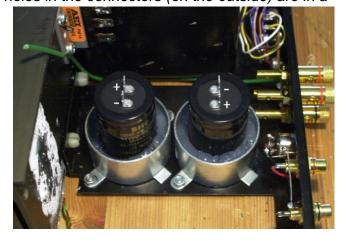
For the inputs we'll use shielded cable between the RCA-connectors and the driver-circuits. It is better to twist all cables that have to be soldered to the same point together before tinning them, it makes soldering a lot easier. See the drawing on page 12 for reference.
