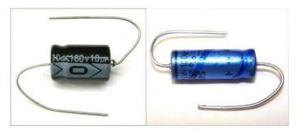
With axial capacitors there is an extra arrow indicating the minus wire, or there is a printed small ring around the body indicating the minus wire. Also the minus wire is direct connected to the aluminum body. The plus wire is sticking through the black plastic cap.
