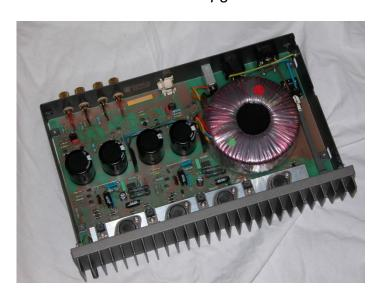
We will replace all electrolytic capacitors, the output connectors, some resistors and capacitors in the input- and DC feedback circuit like Quad did in the 606 MKII, 707 and 909. Some signal capacitors are replaced by high quality capacitors.
