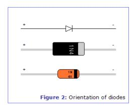
The cathode will be indicated by a white, silver or black line on the body of the diode.
