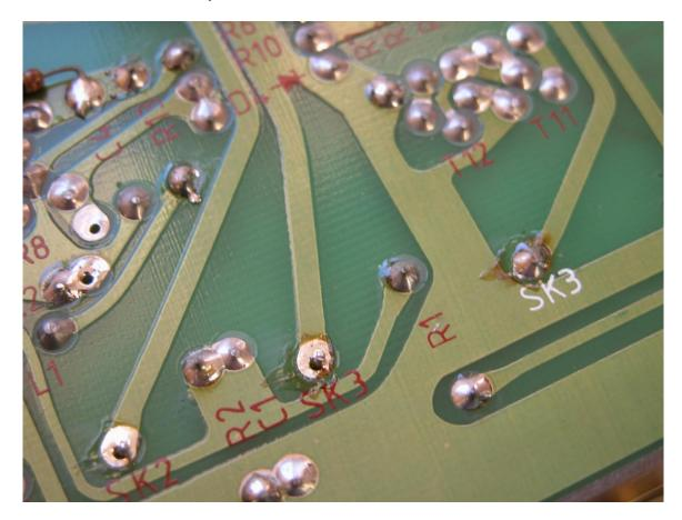
On the back of the boards the component-numbers for the left channel are printed in white, for the right-channel in red. The schematic for both channels is identical but not the object-location.
