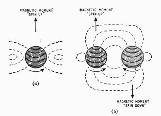
Fig. 1. "Magnetic moments of spinning electrons: (a) unpaired electron; (b) paired electrons.
