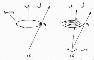
Fig. 3. Precession of an unpaired electron under the influence of external magnetic fields. At (a) is shown the precession with an external steady magnetic field H<sub>0</sub>. A clockwise polarized r.f. field will have no effect. At (b) is the precession under the influence of a steady field H<sub>0</sub> plus an anti-clockwise polarized r.f. field he<sup>jmot</sup>.
