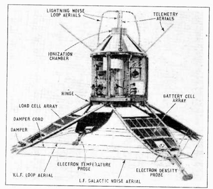
Fig. 1. Overall view of UK3 satellite showing the three loop aerials and other external parts.
