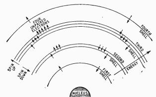
Fig. 2. Shawing the relative energy levels of electrons in an iron atom.
