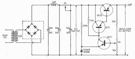
Fig. 4. Power supply unit for the tachometer.
