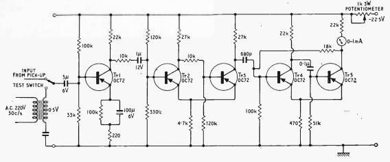
Fig. 3. Complete circuit of tachometer showing Schmitt trigger and standardized pulse generator.
