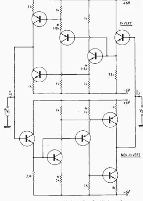
Fig. 4. Simple gyrator. (Below) Fig. 5. High-grade gyrator.
