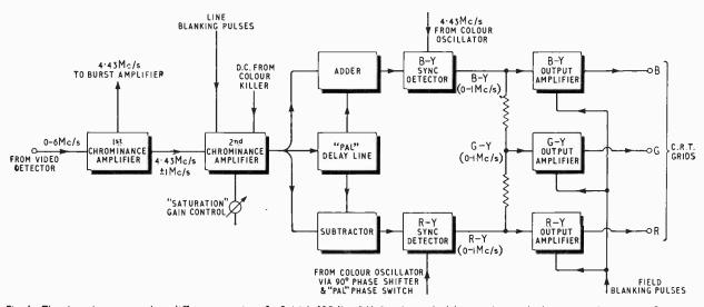
Fig. 6. The chrominance or colour difference section of a British 625-line PAL-D colour television receiver, which extracts the colour information from the composite video signal after the video detector, amplifies it, demodulates it, and reconstitutes (or decodes) the three colour-difference signals to drive the R-Y, G-Y and B-Y picture tube control grids which together with the + Y luminance signals on the cathodes reproduces red, green and blue components of composite picture signal.
