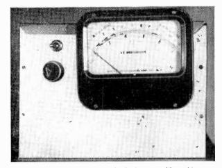
Fig. 6. Complete instrument, with 0-ImA meter calibrated in r.p.m.
