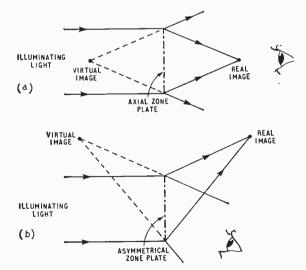
Fig. 3. Offset image at (b) enables separate viewing of real and virtual images.
