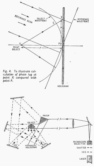
Fig. 5. Apparatus used for producing 3-D Bragg reflection holograms.
