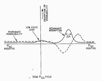
Fig. 4. Microwave absorption and permeabiliy of ferrite as a function of steady magnetic field strength.
