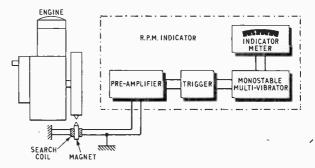
Fig. 1. System used to measure rotational speed of an engine.
