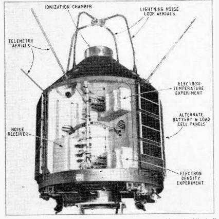
Part of the interior of UK3. Normally the spacecraft is covered with 12 panels of "solar" cells which provide electric power for the vehicle and experiments.
