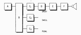
Fig. 1. Block diagram of an electronic organ, A, main oscillators; B, dividers;  $C_1$   $C_2$   $C_3$ , keying systems; D, voicing networks; E, summing system and pre-amplifier; and F, power amplifier.
