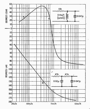
Fig. 4. Phase shift over the normal operating frequency range of two filter circuits.
