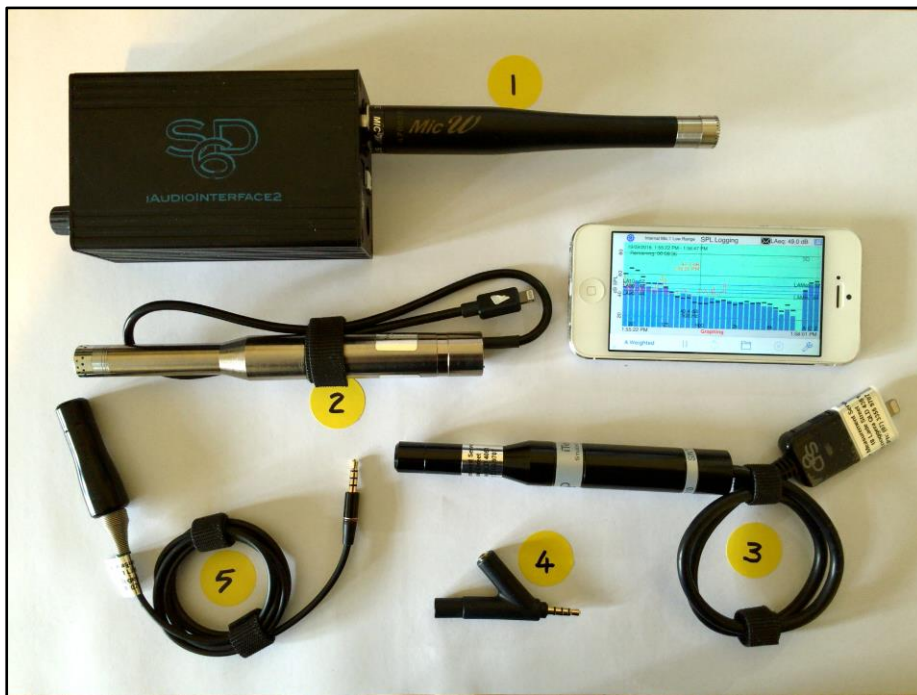
Photo: Apple iPhone with SPLGraph app and external microphones.
