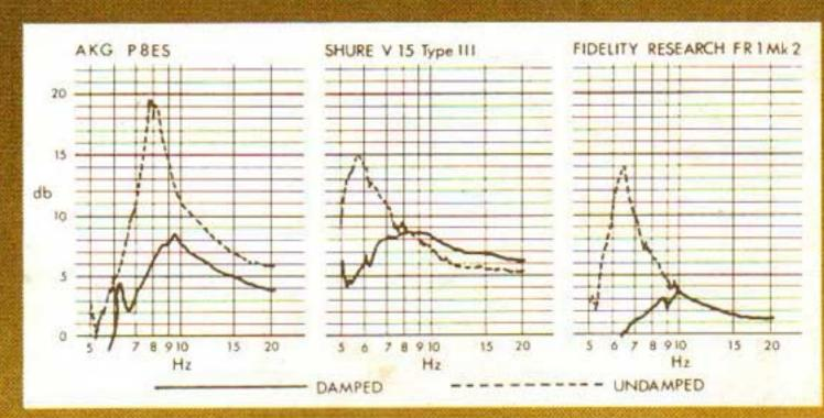
The illustrations show typical extreme low frequency response characteristics of three cartridges in the Series II Improved erm.
