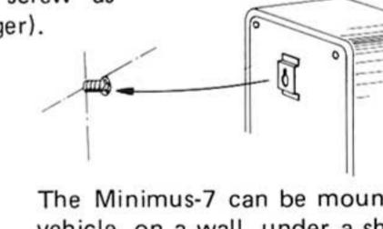
The Minimus-7 can be mounted in a vehicle, on a wall, under a shelf, to a ceiling--using a special bracket (40-2031). See instructions provided with bracket.
