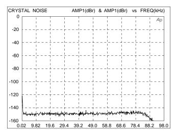
Figure 10. Muted Idle Channel Noise
