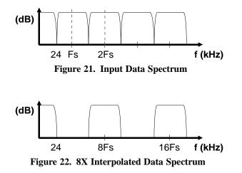
The CS4328 interpolation stage is followed by a sample-and-hold function where the data points from the interpolator are held for eight ( $64 \times$  Fs) clock cycles. The resulting frequency response is a sinx/x characteristic with zeros at  $8 \times$  Fs mul-
