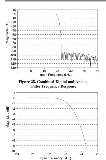
Figure 29. Combined Digital and Analog Filter Frequency Response
