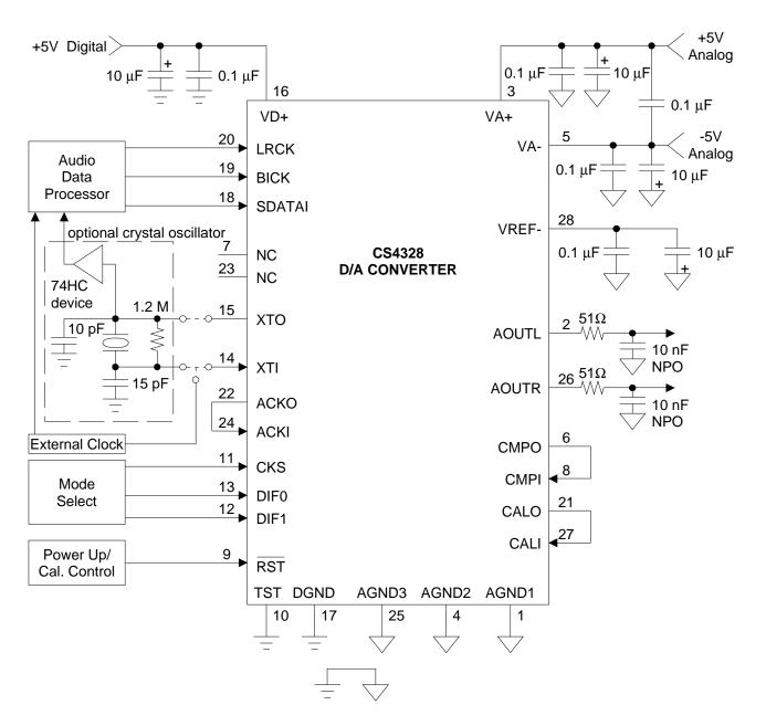
Figure 1. Typical Connection Diagram
