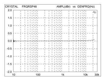
Figure 9. Frequency Response (48 kHz word rate)
