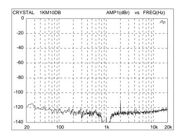
Figure 19. 1 kHz, -10 dB Input FFT Plot
