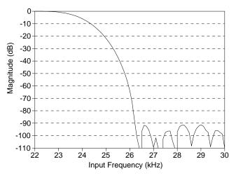
Figure 30. Combined Digital and Analog Filter Transition Band
