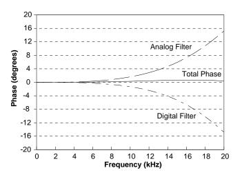
Figure 27. Deviation From Linear Phase
