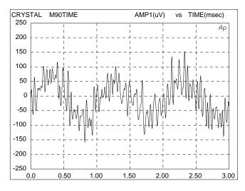
Figure 16. 1 kHz, -90 dB Input Time Domain Plot
