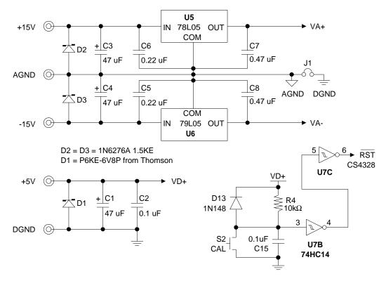
Figure 1. Power Supply and Reset Circuitry
