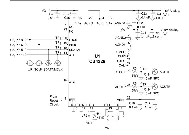
Figure 2. CS4328 DAC Connections
