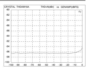
Figure 12. THD+N vs 18-bit Input Signal Level
