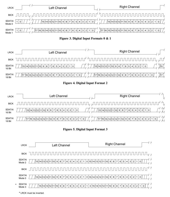
Figure 6. Digital Input Formats 0, 2 and 3 with 16 BICK Periods
