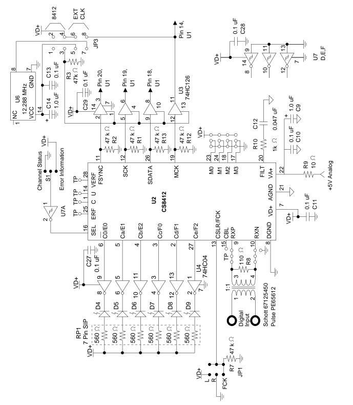
Figure 3. CS8412 Digital Audio Receiver Connections
