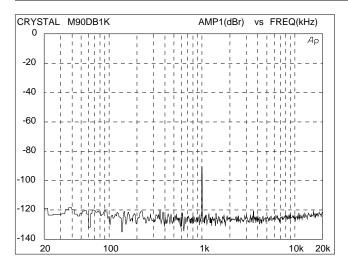
Figure 15. 1 kHz, -90 dB Input FFT Plot
