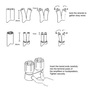
When estimating the length of loudspeaker cable, provide sufficient to enable access and tidy securing. Some cable, is quite heavy and you should be careful to place your cables so that they do not cause undue strain on the binding posts of the amplifier or loudspeaker.
