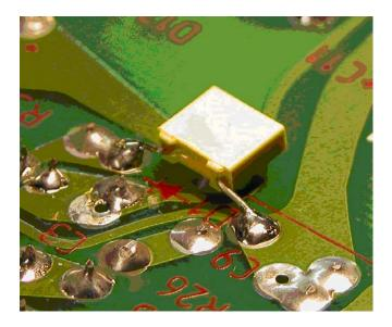
If you want an input-sensitivity of 0 dBm (775 mV), 1mWatt in 600 ohms, which is standard, replace R11 with 12 Ohm. If you leave R11 in place the input-sensitivity will be 500mV. If R11 is replaced with 15 Ohm, the sensitivity will be 1000mV (for professional use).
