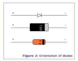
The cathode will be indicated by a white, silver or black line on the body of the diode.
