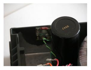
Remove the led circuit board from the front of the amplifier
