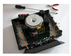
Remove the connectors from the PSU, make notes, or pictures! There is no need for soldering here. There are four large posidriv screws around the transformer, remove those. Be careful, sometimes they are a little bit covered by the transformer.
