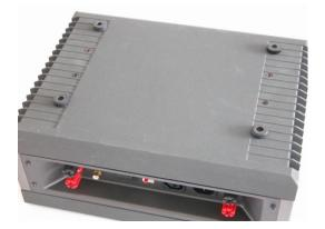
Remove the 8 screws on the bottom and the 4 screws from the rear panel. Remove the bottom and the U shaped chassis part.
