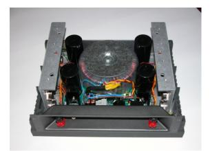
The unit will looks like this. Remove the amplifier boards with a long Philips (posidriv no 2) screwdriver; be careful not to make contact with the components on the boards. Remove (loosen) the connectors on the boards with small pliers. Make notes about the position and the colors, or pictures.
