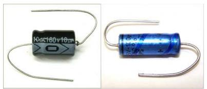
With axial capacitors there is an extra arrow indicating the minus wire, or there is a printed small line (ring) around the body indicating the minus wire. Also the minus wire is direct connected to the aluminium body. The plus wire is sticking through the black plastic cap.
