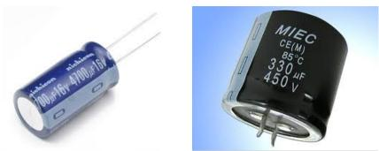
Also if the capacitor has wires, the minus wire is the shortest one!
