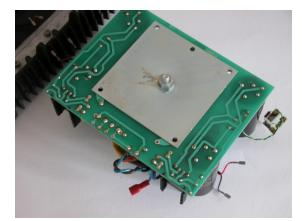
Now the Psu caps can be replaced. The revision of the amplifier boards is not different from the MKI, the MK II has already the input and feedback modification implemented. Rebuilt in reverse order. No need to upgrade the wires in a MKII.
