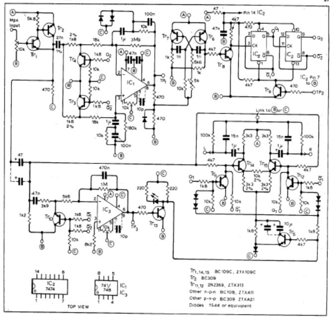
▲ Fig. 14. Modifications to the Portus and Haywood decoder to improve both distortion and channel separation. Faster switching times and high gain transistors in the matrix with a different input amplifier arrangement give IkHz distortion better than 0.04%. Voltage levels of points A, B and C can be either +12, +6 and 0V or +6, 0 and -6V respectively.
