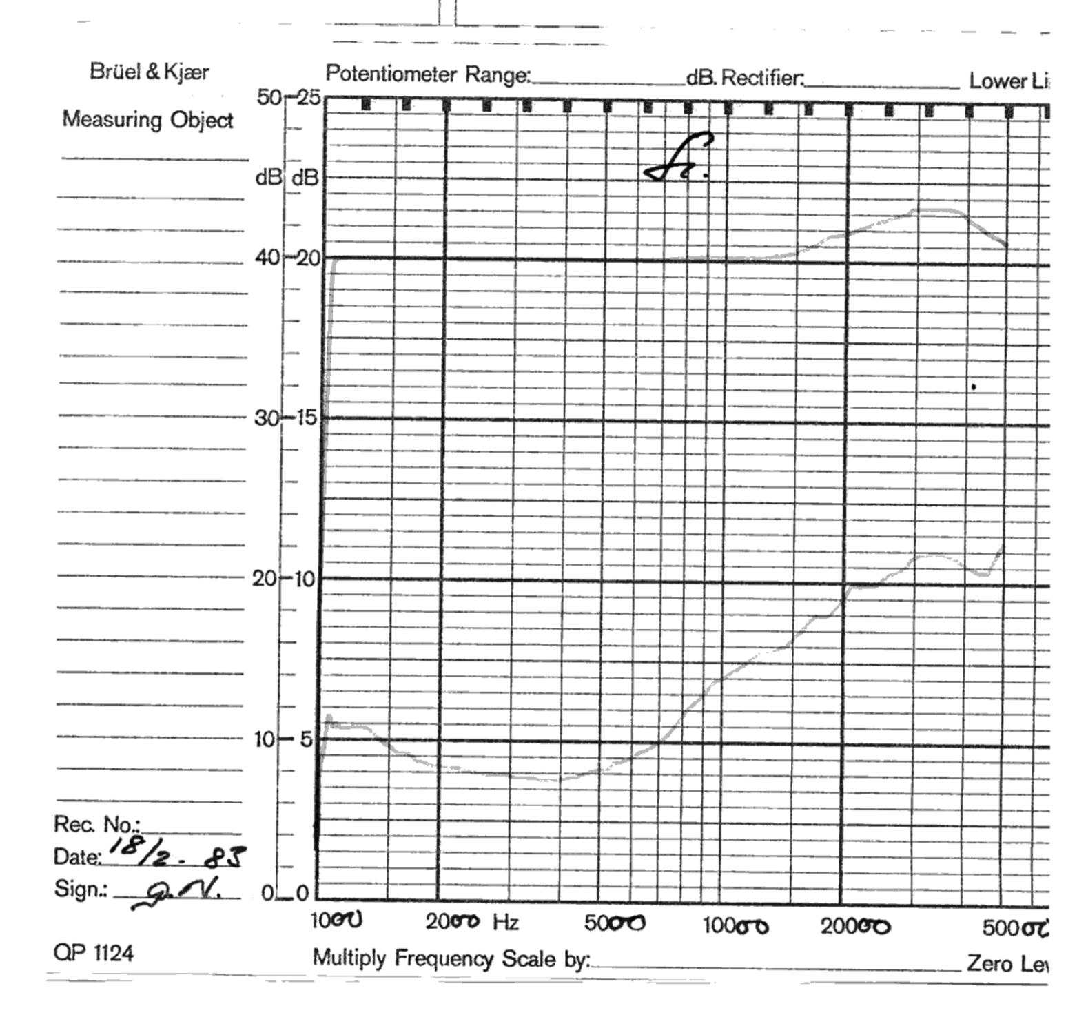
The frequency response and channel separation curves have been measured with the use of Brüel & Kjær Level Recorder type 2307 and Response Test Unit type 4416, with Test Record JVC TRS-1005. Measuring conditions were:
