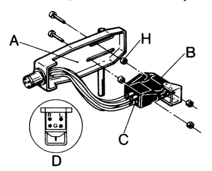
1. The leads from the headshell (A) should be connected to the terminal pins (C) of the cartridge (B) by means of the clips attached to the leads. Please observe the colour code (D), otherwise the channel orientation and phasing of the cartridge will not be correct.
