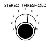
comes worse than this, the tuner automatically switches over to monophonic FM and thus reduces the noise level appreciably. For the home tape recordist, this feature can save a valuable recording from being ruined by interference. The tuner instantly returns to stereo once the disturbance has passed.
