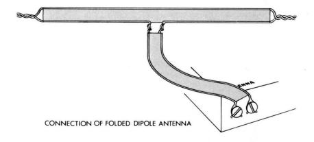
tively as shown above. The dipole should then be opened to a full "T" shape and positioned to give the strongest signal possible on the tuning indicator or meter on the front of the tuner. Tuners using an indicator tube show a strong signal when the dark strip in the center shrinks to its narrowest. Tuners with meters show a strong signal when the pointer is at its highest reading.
