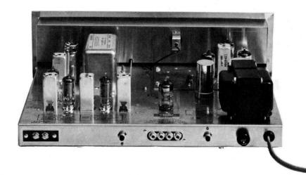
There are two sets of outputs for left channel and for right channel on the rear of your Scott tuner. Connect one of the two audio cables provided from the left channel ( audio or high ) output to the left tuner input on your stereo amplifier. Some amplifiers refer to the left input as Channel A. Connect the remaining audio cable to the right channel (audio or high) output to the right tuner input of the amplifier sometimes referred to as the Channel B input.
