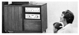
If you install your tuner in the same cabinet with your amplifier, always place the tuner alongside the amplifier or underneath it — never above it, since the amplifier produces much more heat than the tuner. Hot air tends to rise and if the tuner is above the amplifier, the heat generated by the amplifier will cause drift in the tuner.
