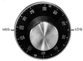
To eliminate this problem, Scott has incorporated a logging scale on the dial as well. This divides the dial into an arbitrary series of numbers from 0 to 100. If you keep a record of your favorite FM stations by their logging numbers, you will not run into problems of confusing one with another. For example, the station at 96.3 megacycles, will log in at 41. The station at 96.7 will log in at 42. Simply tune the station by means of this logging scale and you will avoid confusion.
