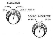
switch to the Monitor position. All stations will become virtually inaudible, and you will hear some hiss in the background. Turn the tuning dial slowly from one end to the other. The moment you hear a steady tone you know you have located a station transmitting in multiplex. Carefully adjust for the cleanest tone combined with high reading on the tuning meter. It is normal for some faint sound to be
