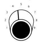
To set the control, first turn it to "O". Tune in between two stations so that the interstation noise is quite audible. Now turn the squelch control clockwise until the noise disappears. Turn the control just a little beyond this point and leave it there. As you tune across the dial, you will find that stations pop in and out from a background of complete silence. A pilot light on the 310 series lights up when the squelch circuit is in operation.
