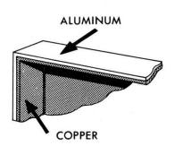
Instead of inexpensive steel chassis, Scott uses electrolytic aluminum with copper cladding in the critical IF and multiplex sections. Copper is a far better conductor than steel and eliminates the losses ordinarily associated with that metal. Aluminum, being non-magnetic, tends to reduce hum and noise, giving Scott tuners an exceptionally high signal-to-noise ratio.
