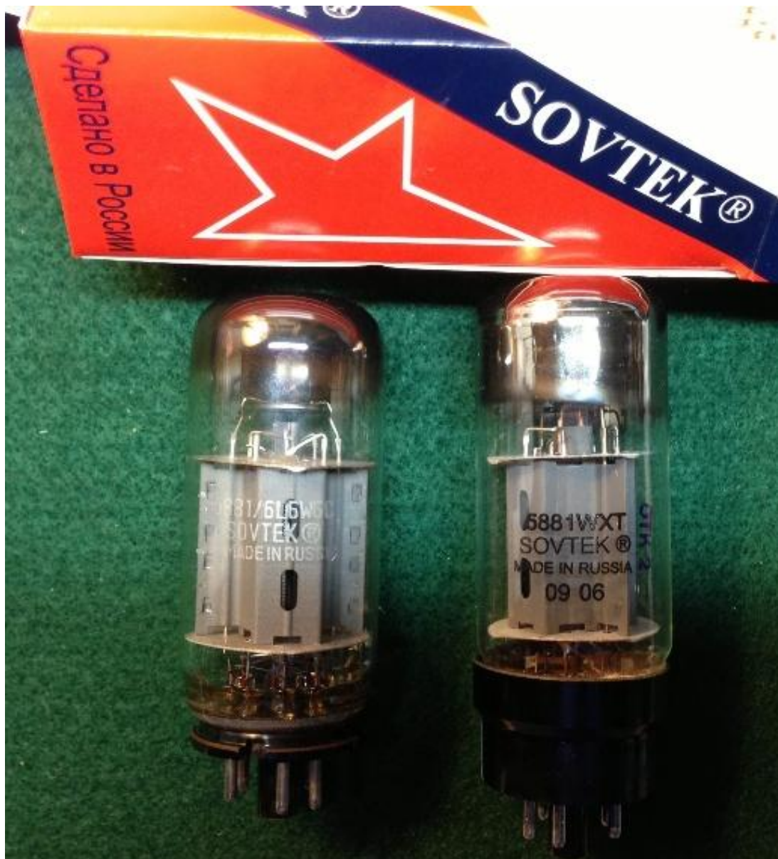
SE-40 Factory tube on Left with coin base, Same tube with a standard base on the right but marked differently
