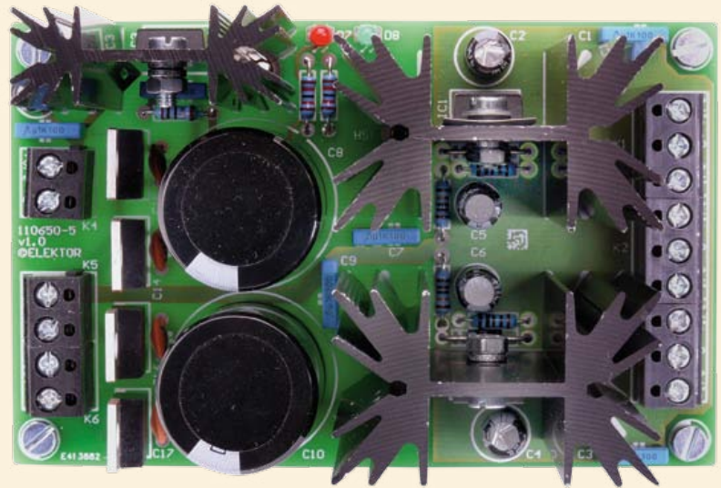
Figure 12. Preamplifier PSU board assembled by Elektor Labs.
