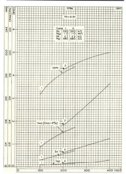
PERFORMANCE OF EF86 AS PENTODE CONNECTED R.C. COUPLED AMPLIFIER PLOTTED AGAINST LINE VOLTAGE, FOR  $R_u\!=\!220~k~\Omega.$
