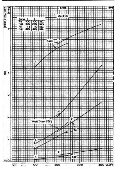
PERFORMANCE OF EF86 AS PENTODE CONNECTED R.C. COUPLED AMPLIFIER PLOTTED AGAINST LINE VOLTAGE, FOR  $R_{\rm B}{=}100~k\,\Omega$
