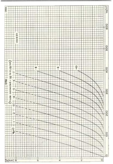
ANODE CURRENT PLOTTED AGAINST ANODE VOLTAGE WITH GRID VOLTAGE AS PARAMETER, WHEN CONNECTED AS A TRIODE
