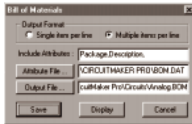
Figure 7.1. You can save, display, or print a Bill of Materials in one of two formats.
