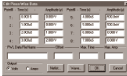
Figure 6.44. Use this dialog box to set the parameters of the piecewise linear waveform.
