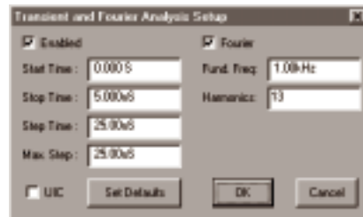
Figure 6.18. Use this dialog box to set up a Fourier Analysis.
