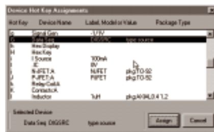
Figure 4.3. Use this dialog box to assign or reassign HotKeys to devices.
