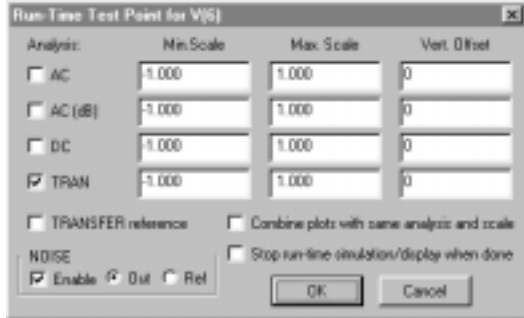
Figure 6.22. Use this dialog box to set up Run-Time Test Points for a Noise Analysis.
