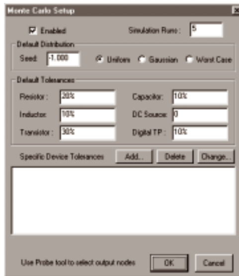
Figure 6.27. Use this dialog box to set up Monte Carlo Analysis.
