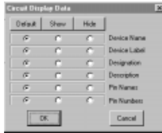
Figure 12.3. Use the Circuit Display Data dialog box to temporarily override the display settings of every device in the circuit.
