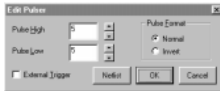
Figure 5.5. Use the Edit Pulser dialog box to change pulse ticks and set free run or external trigger mode.
