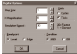
Figure 5.4. Use the Digital Options dialog box to control the size of a step and other digital simulation options.
