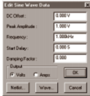
Figure 6.40. Use this dialog box to edit sine wave data.
