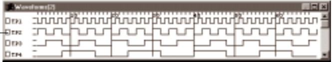
Figure 5.3. The Waveforms window lets you graph the states of nodes over time as the simulation runs.
