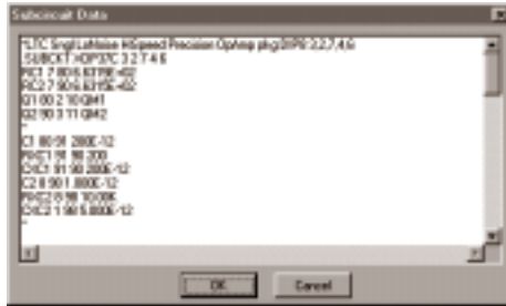
Figure 16.14. Use this dialog box to edit or view an existing subcircuit.
