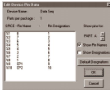
Figure 4.9. Use this dialog box as a reference for pin SPICE information.
