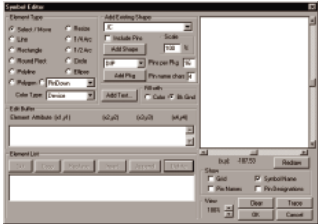
Figure 16.1. Use the Symbol Editor to create or modify schematic symbols.
