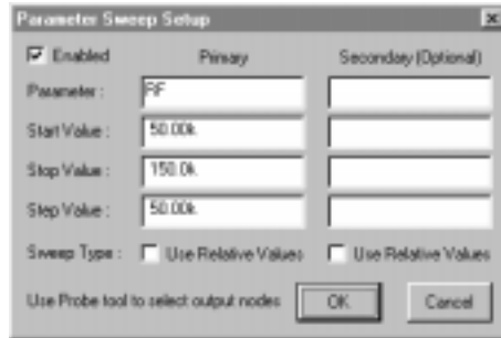
Figure 6.16. Use this dialog box to set up a Parameter Sweep Analysis.
