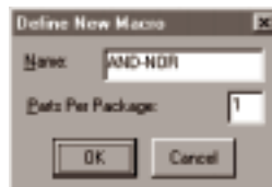
Figure 16.4. The name you enter here is used later to select the device from the library.
