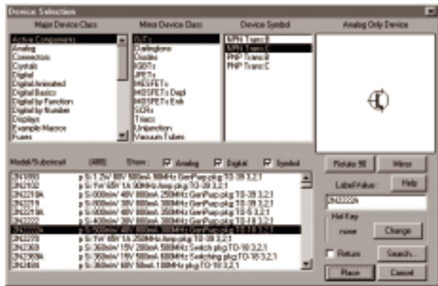
Figure 4.2. The Device Selection dialog box lets you graphically browse and select from a library of several thousand devices.
