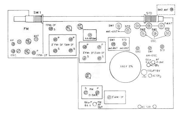
through a  $0.1\,\mu\text{F}$  capacitor, with the iron core of the IF series-resonant wavetrap screwed all the way out. The signal is measured at the top of the potentiometer, and the circuits should be tuned for maximum response and symmetrical curve-form. The IF signal should thereafter be applied through the aerial jack and the IF series-resonant wavetrap tuned for maximum attenuation.
