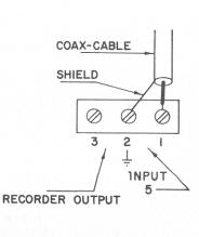
Channel 5 connections are just below the inputoutput terminals (see photograph). This is a high level input for use with line level signals, tape machine outputs, tuner outputs, high level ceramic phono cartridge outputs or other signals of .02 volts or more. It is a grounded input. If line isolation is required, a repeat coil such as the 15036 or the 15095 line transformer must be mounted externally.
