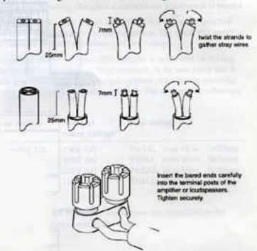
When estimating the length of loudspeaker cable, provide sufficient to enable access and tidy securing. Some cable is quite heavy and you should be careful to place your cables so that they do not cause undue strain on the binding posts of the amplifier or loudspeaker.
