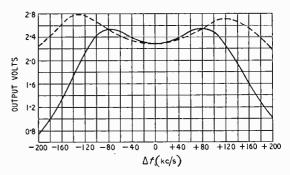
Fig. 7. Potential derived from discriminator to feed tuning indicator (solid line); ImV constant input to receiver. Dotted line shows response of discriminator alone.
