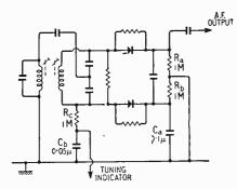
Fig. 6. Circuit modifications to obtain tuning indicator drive from discriminator.
