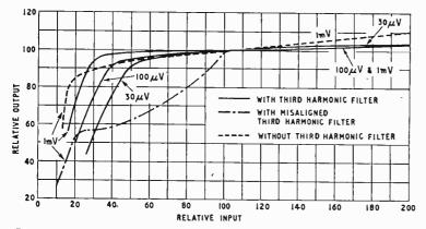
Fig. 4. Correct dynamic-limiter characteristics for various input levels and effect of mis-tuned harmonic filter (two-kneed curve) and absence of filter (dotted curve).
