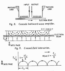
Fig. 10. Electron motion in crossed fields.
