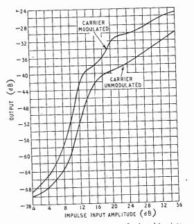
Fig. 14. Input/output characteristic for impulsive interference. Input carrier level  $5C0_{\mu}Y$ , impulse p.r.f. 2,500/sec; relative output is referred to output with  $\pm 35kc/s$  deviation at 2kc's and impulse input amplitude is referred to  $1\mu V$  peak per kc/s bandwidth.
