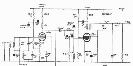
A circuit for an i.f. strip using the new frame-grid variable-mu EF183 is shown. It consists of a first i.f. stage which is common to sound and vision, followed by a second i.f. stage in each channel. Apart from component value changes, the only difference from normal practice is the use of  $\pm 10\%$  neutralising capacitors. When the strip is used with the frame-grid PCR89 mixer, adequate gain is achieved for use in fringe areas without the addition of a further vision i.f. stage.
