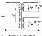
Fig. I Relative instantaneous voltages in a transformer is shown by arrows.
