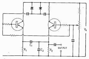
Fig. 6. Transistor-oscillator circuit (equivalent to Fig. 3).
