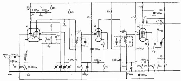
Fig. 1. Theoretical circuit diagram of receiver incorporating new limiter.
