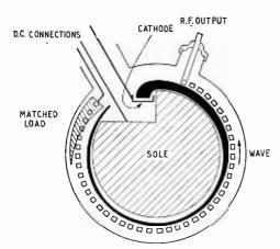
Fig. 15. Crossed-field backward-wave oscillator.
