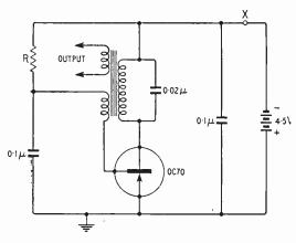
Fig. 1. Transistor oscillator circuit using triple-wound transformer.
