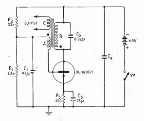
Fig. 3. Oscillator circuit with base current stabilized.
