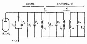
Fig. 3. Equivalent circuit of limiter and discriminator.
