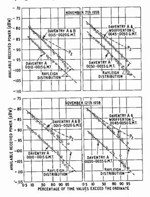
Fig. 3. Distribution of signal envelope amplitude.
