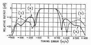
Fig. 5. Tuning characteristic with (a) narrow-band discriminator, (b) wide-band discriminator.
