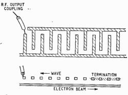
Fig. 7. Interdigital line backward-wave oscillator.
