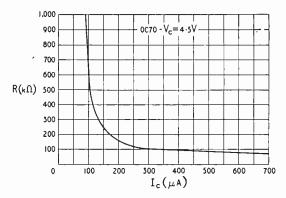
Fig. 2. Collector current with different values of resistor R.
