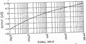
Fig. 13. Variation of a.f. output with input level. Output is referred to ImV and input level is open-circuit voltage from 75- $\Omega$  source.
