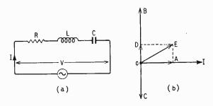
Fig. 1. A typical a.c. circuit diagram and corresponding vector dicgram. What are all the arrow-heads for?
