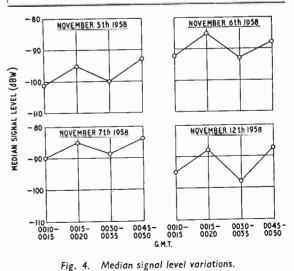
Boulder Laboratories, National Bureau of Standards, U.S.A. † From information obtained antenna gains were almost identical at 20dB with reference to a dipole in free space. Transmitter outputs were not the same, however, some being 50kW others 70kW. Ed.
