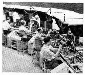
TAILOR-MADE gravity convevors constructed from Dexion slotted angle and "Glidewhee's" are being used on the television receiver assembly line at the Southend-on-Sea factory of E. K. Cole Ltd.
