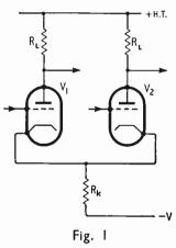
values, with equal loads,  $R_L$ , and similar mutual conductances, have a common cathode resistor  $\mathbf{R}_{\mathbf{k}}$ . For the correct functioning of the circuit it is necessary for the cathode current (i.e., the total valve currents) to be as nearly constant as possible and independent of any changes caused by varying inputs to the grids. To achieve this, one end of R<sub>k</sub> is taken to a large negative voltage and
