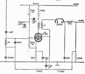
to take the conventional EF80, with the EF183 retained in the first i.f. stage. With this new line-up, a 2.0V video output is obtained with  $9\mu V$  on Band III and  $5\mu V$  on Band I.
