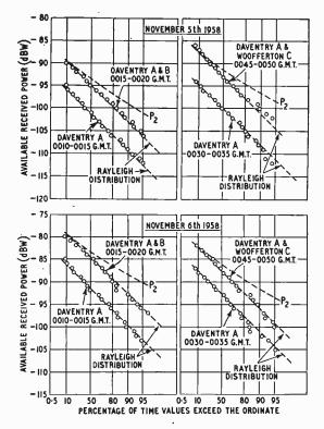
Fig. 2. Distribution of signal envelope amplitude.
