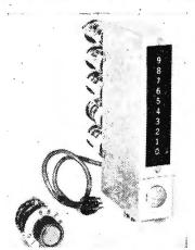
allows the selection of a digit between 0 and 9, but several of the devices can be connected in cascade to count units, tens, hundreds, thousands, etc., and the same method of pre-selection is applied to them all. A rotary switch at the end of a fivewire cable is used for the remote pre-setting of each decade.
