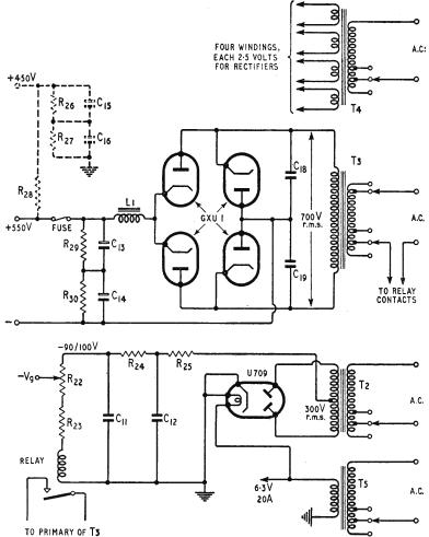
Fig. 2. Power supplies for 400-watt amplifier.
