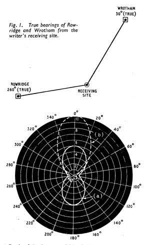
Fig. 2. Polar diagrams of (a) a halfwave dipole and (b) a 3-element Yagi.
