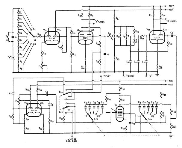
Fig. 3. Amplifier and time-base circuits.
