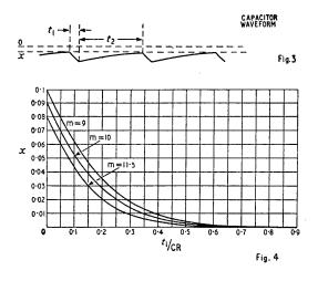
Figs. 2 and 3 respectively. Referring to these figures, we will let the voltage on the capacitor at the end of the period  $t_2$  be x, then the amplitude of the effective charging voltage during the line pulse  $t_1$  will be 1 - x, the capacitor charging up according to the relation
