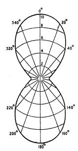
Fig. 4 shows the optimum orientation of the aerial to achieve this performance. It reveals that if a dipole were used, or an aerial with a similar polar diagram and relative position of the elements, then the plane of the elements in this aerial must be on a line running from 145° to 325°. When laying out this bearing with a compass due allowance must be made for the magnetic deviation. Át present this is 9° west at the site of the receiver, so that 9° must
