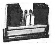
CQ amplifier showing (above) mains transformer and grainoriented output transformer and (below) controls on the die-cast pre-amplifier panel.
