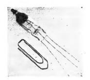
1.32in long and 0.39in in diameter. The electrical tolerances are slightly wider than those normally met in cold-cathode tubes, but the makers say this is offset by the long life, reliability and low cost of the tube. The anode hold-off voltage is 310V, while the trigger striking voltage is 170V. The operating current limits are 3mA to 9mA, and at 4.5mA the anode-cathode voltage lies between 95V and 140V.
