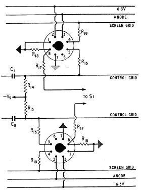
Fig. 5. Preferred layout for output stages.
