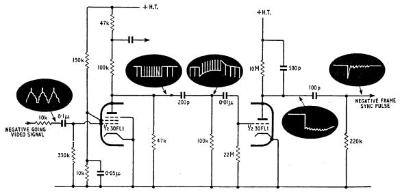
Fig. 10. Complete circuit diagram of the improved frame pulse separator, based on a double valve.
