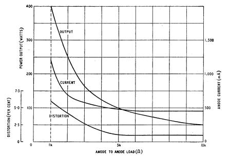
Fig. 3. Performance of amplifier for various anode loads.
