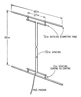
Fig. 7. Simple two-element stack using T-matched dipoles.
