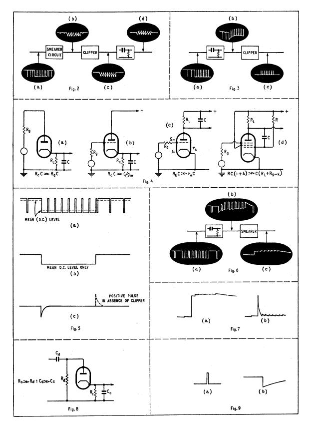
entiation is the first operation, using a critical timeconstant RC network. The use of such a network is well known and forms the basis of a large group of sync separators. For the British system the maximum difference obtainable between line and frame pulses is 47% of the line pulse amplitude, and is produced with a time constant of  $21.6\mu$ sec.
