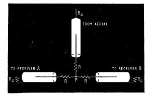
Fig. 1. A splitting network to avoid reflections.
