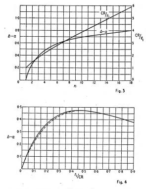
require the maximum difference between the amplitude of the first half line pulse, b, and the amplitude of the overshoot of the line pulses, a, in order to give the greatest latitude in clipping level. The amplitudes a and b are given by the voltage rise on the capacitor during the intervals  $t_1$  and  $t_3$ , i.e.
