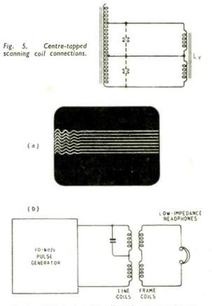
Fig. 6. At (a) is shown the effect of velocity modulation of the frame scanning current waveform, while (b) shows a method of null adjustment for minimum coupling between the line and frame coils.
