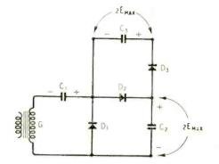
Fig. 10. First stage in the extension of the Fig. 7 technique to higher voltages on its own.
