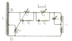
Fig. 7. Width and form controls added to scanning coil circuit.
