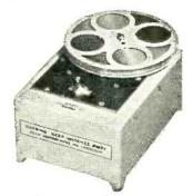
Plessey "Cascap" miniature ceramic capacitors and (right) Leevers-Rich bulk eraser for small magnetic tape reels.
