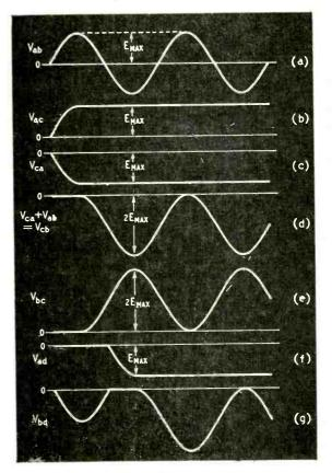
Fig. 2. Starting-up waveforms of the various voltages in Figs. I and 3 on no load.
