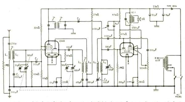
Circuit diagram of the 2-valve Superheterodyne receiver described in the text.  $C_5$  is a small capacitor to be found experimentally.
