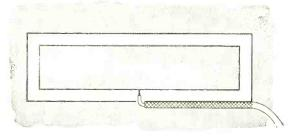
Fig. 6. Folding a slot reduces its impedance. The method of attaching a low-impedance feeder is shown here.
