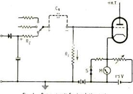
Fig. 4. Basic circuit for insulation test.
