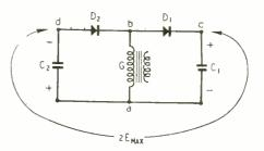
Fig. 3. First kind of voltage doubler circuit, formed by working a second rectifier unit in parallel with the same source.
