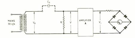
Fig. 1. Basic circuit for capacitance measurement.
