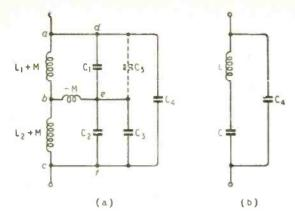
Fig. 3. Equivalent circuits of scanning coils.
