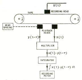
Fig. 6. Simplified schematic of an auto-correlation analogue computor using a magnetic tape system to obtain the necessary time lags. The recording meter prints the values of successive integrals (one for each time lag) as a series of vertical lines of varying height.
