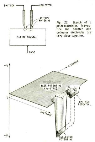
Fig. 24. A surface representing potential levels in the point transistor. Provided that the points are very close together the "barrier" between the emitter and collector is somewhat lower than the general potential level of the base as a whole. This makes it more likely for most of the emitter current to find its way to the collector.
