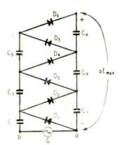
Below : Fig. 13. The first two half cycles of operation of a "working model" based on Fig. 12.
