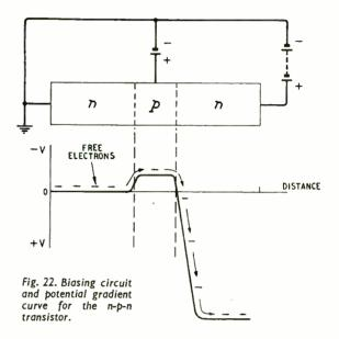
The width of the layer is thus a critical factor in deciding the intrinsic gain of a transistor. Control of the width of this layer to such very small dimensions is one of the most difficult problems which manufacturers have to solve.
