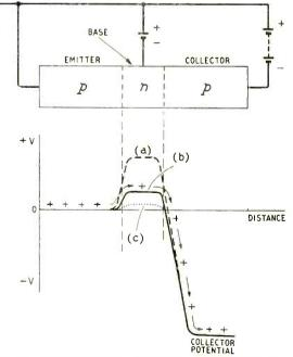
Fig. 18. Biased transistor. The full line (b) represents the normal d.c. negative bias on the base. The broken line (a) shows the effect when that bias is removed and the dotted line (c) shows what happens when the bias is increased.
