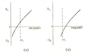
Fig. 4. Reactance sketches for equivalent circuits in Fig. 3: (a) circuit abed and (b) circuit befe.
