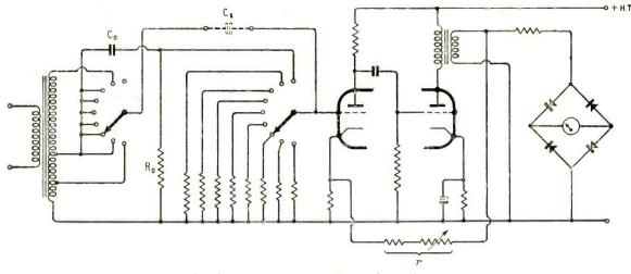
Fig. 2. Capacitance range switching and amplifier circuit.
