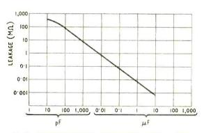
Fig. 3. Permissible leakage resistance for reading accuracy up to +5% in capacitors of different values.
