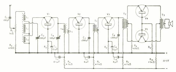
Fig. 2 Circuit diagram of transistor receiver. Details of coil and transformer windings are given in the table on the following page
