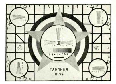
Colour test card for the experimental station. The fivepointed star is red, while the three circles are blue, yellow and green respectively. The quartered square in the middle is also made up from these four colours. (Reproduced from the Soviet journal Radio.)
