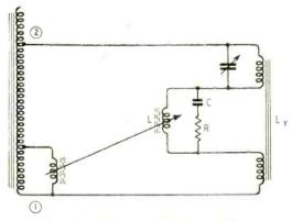
Fig. 8. Alternative position for series width coil.
