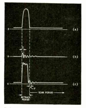
Fig. 2. Voltage waveforms in VI anode circuit of Fig. 1: (a) potential across VI anode transformer windings; (b) across leakage inductance  $L_4$ ; (c) combined potential cpplied to VI anode.
