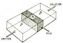
Fig. 16. Sketch of p-n-p junction transistor showing electrodes.
