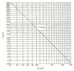
Fig. 4. Calibration curve for inductance scale (C\_8) using a frequency of 1 Mc s.
