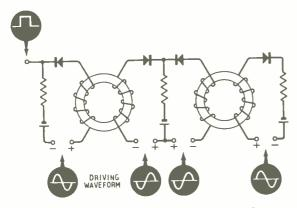
Fig. 3. Magnetic amplifiers connected in series to form a delay line. Each of the two stages delays the input pulse by one half cycle of the driving waveform.
