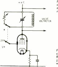
Fig. 1. (Left) Basic circuit for measurement of dynamic resistance.
