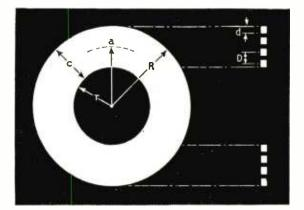
Simplified sketch of printed coil, showing meaning of abbreviations used in the Appendix and in the captions to Figs. 3, 4 and 5. (a=mean radius, r=inner radius, R=outer radius, c=depth of winding, d=width of conductor, D=pitch of winding.)
