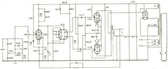
The values of the cathode resistors in the output stage are 270  $\Omega$  for "normal" loading Circuit of Mullard " 5-10 " amplifier. and 437  $\Omega$  for "low loading". Feedback resistor and capacitor values depend on the output impedance of the loudspeaker used.
