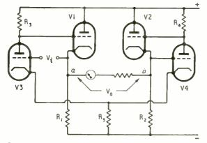
Fig. 1. Outline circuit of stable impedance "transformer" with I : I voltage ratio, which forms the basis of Fig. 4.
