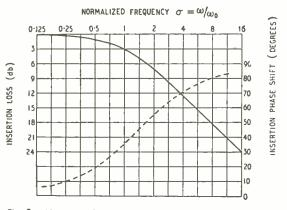
Fig. 2. Normalized insertion loss and phase shift character-istics for a "first-order" filter.
