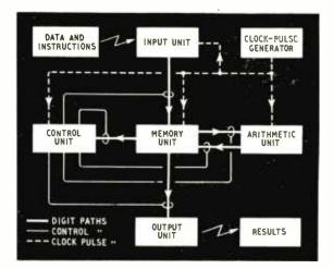
Fig. 1. Block diagram of a general-purpose digital computor, showing various functions of the memory unit.
