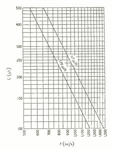
Fig. 3. Calibration curves for frequency scale (C<sub>1</sub>) using 117 and 170- $\mu$ H coils.
