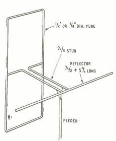
Fig. 4. A reflector can be mounted behind a skeleton slot in the manner shown here. Note this reflectar is at right angles to the long sides of the slot.
