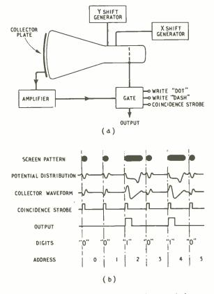
Fig. 8. Electrostatic storage system using a cathode-ray tube (a) with the associated waveforms representing digits at (b).
