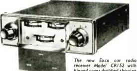
receiver Model CR152 with hinged cover dropped showing the three tuning drums.
