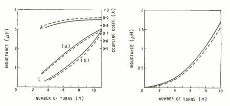
Inductance (L) and coupling coefficient (k) of printea coils with d=0.25 mm Fig. 3 (left). and D=1.025 mm. Full lines are calculated values and broken lines measured values. In curves k and (a), R is constant at 16 mm and r is variable; in curve (b) r is constant at 6 mm and R is variable.
