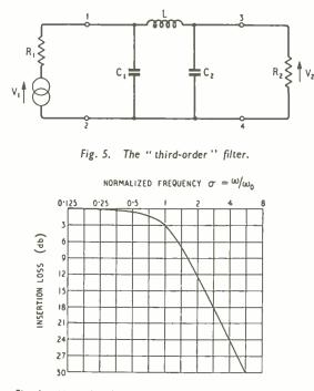
Fig. 6. Normalized insertion loss for a "third-order" filter of "maximal flatness".
