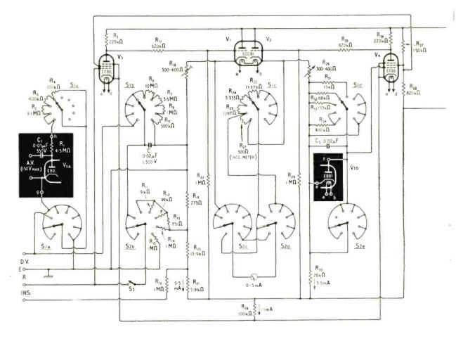
Fig. 4. Complete circuit diagram of electronic test meter. The alternative probe for the higher range of a.v. is shown in the
