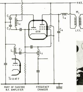
Section of the printed circuit (frequency changer) with corresponding section of the circuit diagram, indicating coils and capacitors which are actually printed. ing the chassis and connector together. The arrangement is seen on the left-hand side of Fig. 1.
