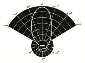
Fig. 6. The cddition of a reflector to a skeleton slot gives it unidirectianal properties and impraves the gain.
