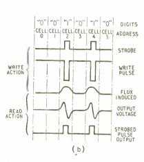
Fig. 6. Magnetic-drum storage, with (a) recording and reading arrangement and (b) waveforms representing the stored digits.
