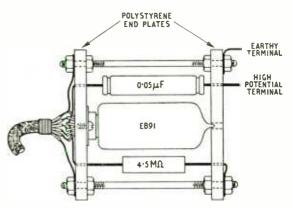
Fig. 5. Simple type of EB91 probe for voltages not over 150 r.m.s. A screening cover should be provided.
