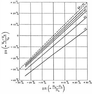
Fig. 5. Diagram showing the percentage departure from voltage balance  $(\delta V)$  in terms of the percentage difference between  $R_{a}$  and  $R_{5}$  ( $\delta R$ ), for several values of amplification, M.
