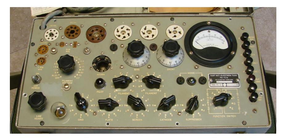
Note the skirted dials on the Bias and Shunt controls. Later variants had number settings engraved in the panel. Except for the first Navy run by Hickok in 1952, all U's were made by Supreme Instruments, company bought by Hickok in 1956.
