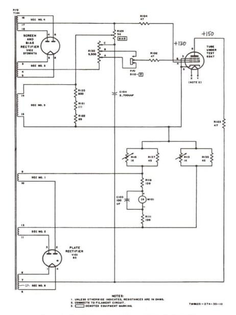
Figure 11. Simplified mutual conductance test circuit, TV-7D/U.
