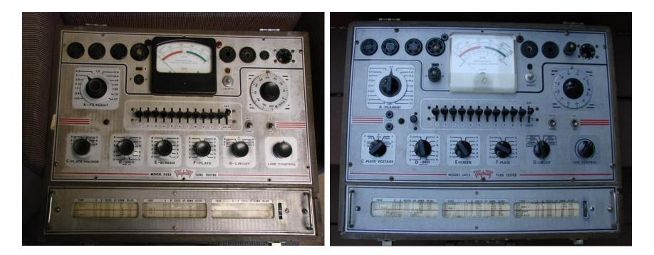
**Both versions identical electrically in the gm test - "Proportional Transconductance"** Because of the meter and leakage test, the "sweet spot" is 2255 to 3000
