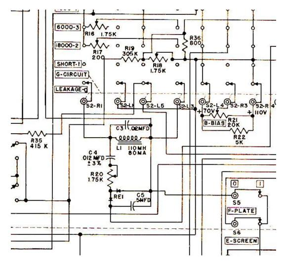
GM signal acquisition and Bias portion of the Schematic
