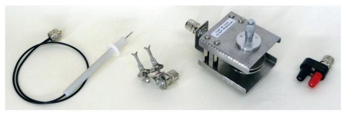
Shown above are a variety of homemade adaptors which can be connected to the UNKNOWN jack on the front panel. The largest one (second from the right) is a variable space capacitor for measuring permittivity – the degree that an insulating material increases capacitance between the plates over the capacitance obtained with air or vacuum spacing.
