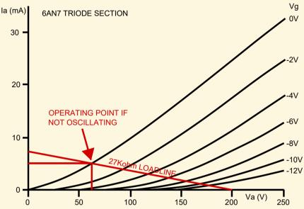
Figure C: plot of the 6AN7's anode voltage versus anode current for various grid bias amounts. The  $27k\Omega$  is the load connected to the plate of the 6AN7 (R2 in Figure A).
