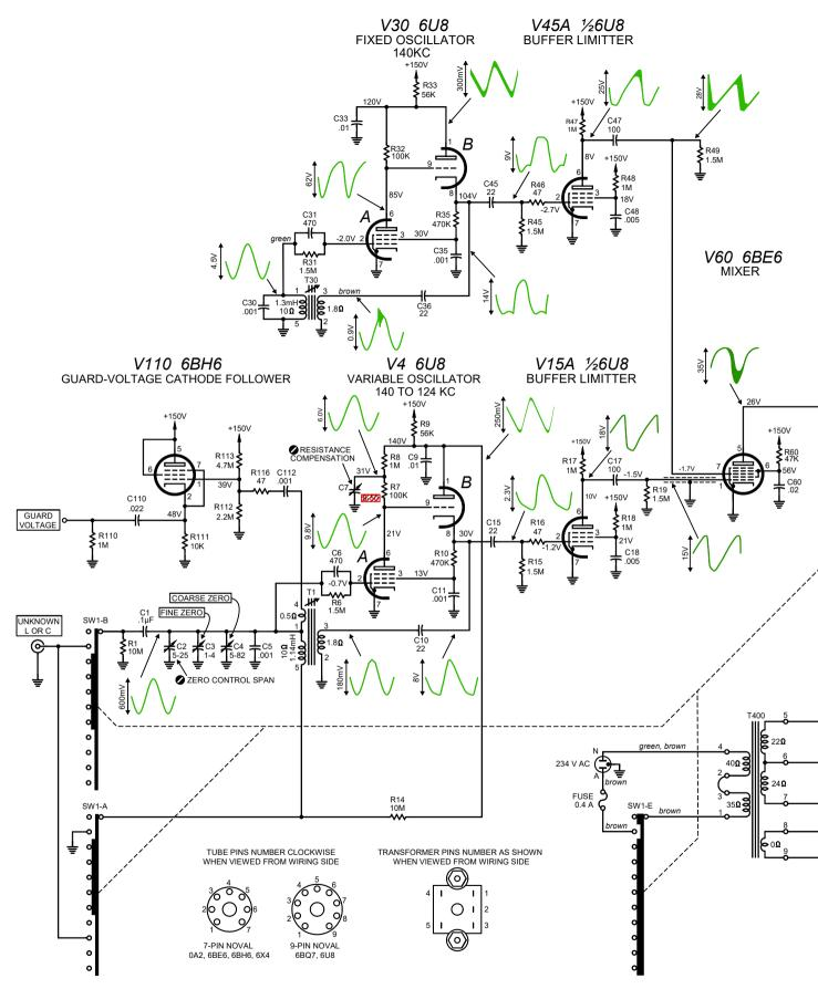
Fig.2: complete circuit diagram for the Tektronix T-130 LC meter.
