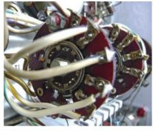
This socket connects to the RANGE SELECTOR on the front panel. The visible ring connects to V70's anode, and the crimped lugs of the ring on the other side connect to the 230V AC mains input.
