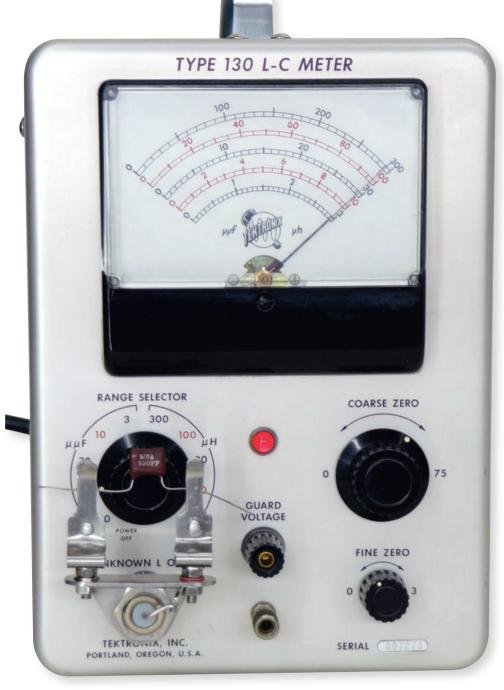
Shown above is the T-130 testing an MSA 100pF capacitor, which returned a reading of ~98pF. Below is a short description of the controls on the front panel: <u>RANGE SELECTOR</u>: an 11-position switch (five each for capacitance and inductance), which also functions as the power switch. <u>COARSE ZERO</u>: used to adjust for capacitance in connecting leads or
