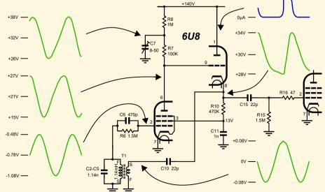
Figure D: the variable oscillator configuration used in the T-130 uses a 6U8 triode pentode.
