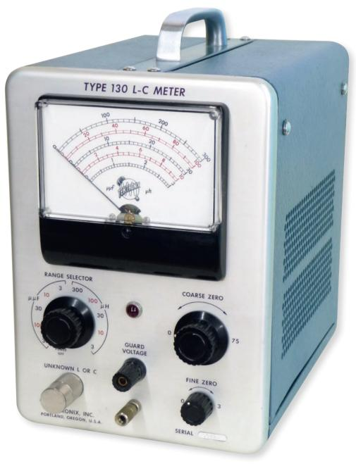
**The T-130 LC meter from Tektronix** was built from 1954 until 1975 and has five capacitance measuring ranges (3pF, 10pF, 30pF, 100pF and 300pF) with 1% FSD accuracy and a stable zero. Thanks to its 4.5-inch (~11.5cm) meter, it can easily resolve down to 0.05pF. It also has five inductance ranges from 3µH through to 300µH.
