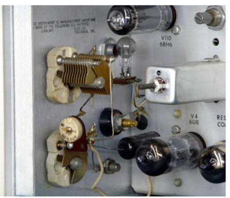
A close-up of part of the variable oscillator section, incorporating V4 and variable capacitors C2-C5, as described in the panel labelled "An ingenious oscillator design".
