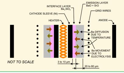
Note that although the tube may test low for gm, its emission can be entirely normal.
