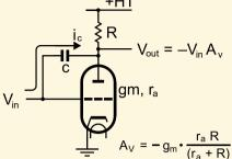
For typical triodes in typical circuits, Av is around -10 to -40. The capacitor then sees a voltage across it of  $(V_{IN} + A_V \times V_{IN})$ , ie,  $V_{IN} \times (1 + A_V)$ , and its
