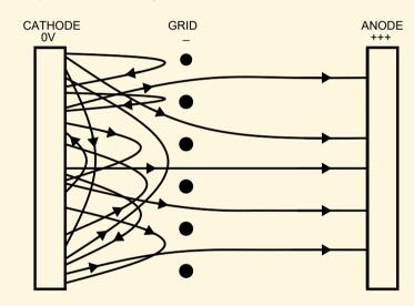
cathode and grid is called a "space charge" and tends to self-limit in local density, as space charge electrons repel more electrons leaving the cathode.
