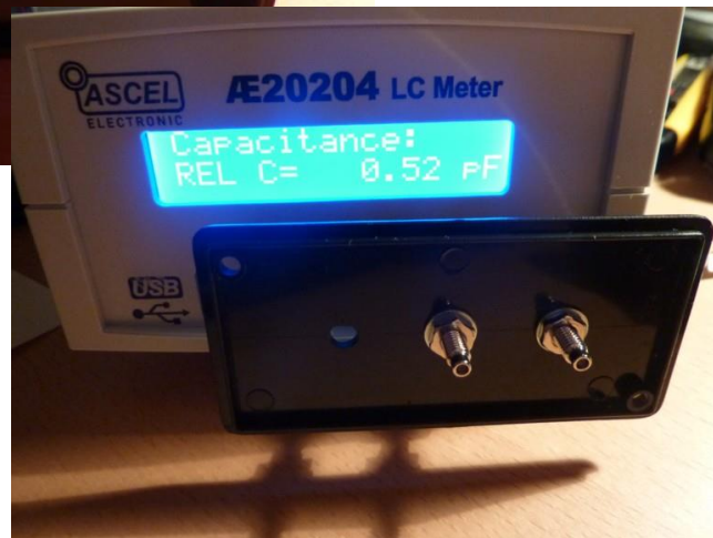
Pictures 3, 4: Testing Teflon-washers for parasitic capacitance – no improvement over standard steel washers and ABS plastics
