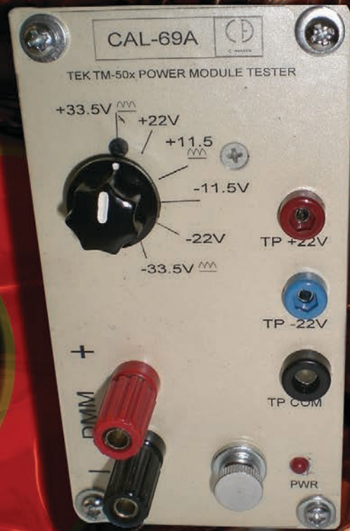
Photo 1: The front panel controls for my CAL-69A power module tester include a power supply selection switch, two reference test points, DMM connection jacks, a test point common, and a LED power indicator.
