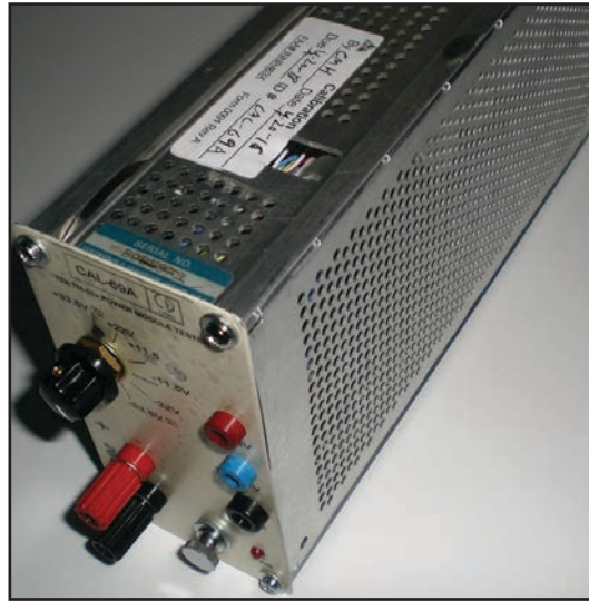
Photo 9: This is the completed, calibrated CAL-69A power module tester.
