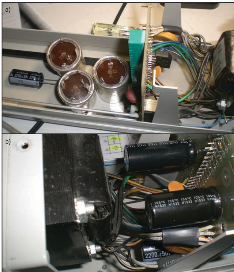
Photo 2: The Tektronix TM501A is shown with three Sprague metal can capacitors removed from the module (a) and the three new replacement capacitors installed on the TM501 PCB (b).
