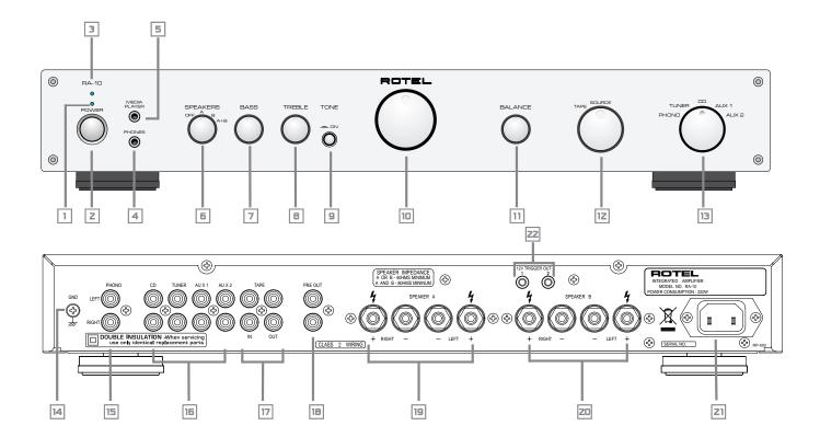
Figure 2: Preamp Input and Speaker Output Connections
