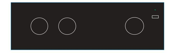
Modified Radford ZD22 front-most panel showing it has just the two new input sensitivity (balance) and volume control potentiometers/knobs, existing on/off switch and new indicator LED. The more substantial aluminium front carrier extrusion having been drilled to accept the new potentiometers.
