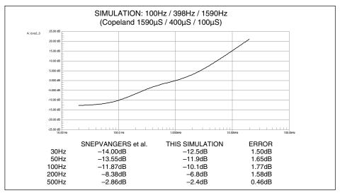
Figure 6. Simulation for 100Hz, 389Hz and 1590Hz (1590µS, 400µS and 100µS), a combination suggested by Copeland. Errors are less than 2dB.
