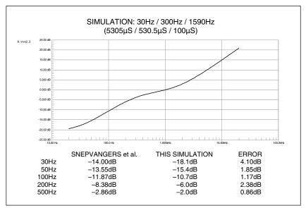
**Figure 4**. This curve was generated by a computerized circuit simulation model using turnover frequencies of 30Hz, 300Hz and 1590Hz, corresponding to time constants of 5305µS, 530.5µS and 100µS. The table compares the results with the data derived from the Snepvangers graph. This combination deviates significantly from Snepvangers' graph.
