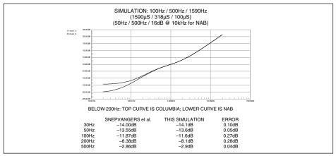
**Figure 8.** Simulation for 100Hz, 500Hz and 1590Hz (1590µS, 318µS and 100µS), as suggested by Eargle and others. This combination produced the lowest errors when compared to Snepvangers' graph indicating, beyond a reasonable doubt, that these are the correct turnover frequencies and time constants for the Columbia Lp equalization curve.
