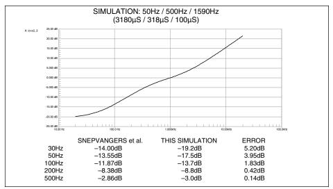
Figure 5. Simulation for 50Hz, 500Hz and 1590Hz (3180µS, 318µS and 100µS). Errors at the lowest frequencies are significant.
