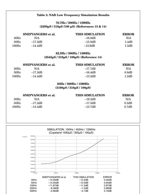
Figure 7. Simulation for 100Hz, 455Hz and 1590Hz (1590µS, 350µS and 100µS), which is Copeland's interpretation of a graph published by Langford-Smith. The results are extremely close to Snepvangers' graph.
