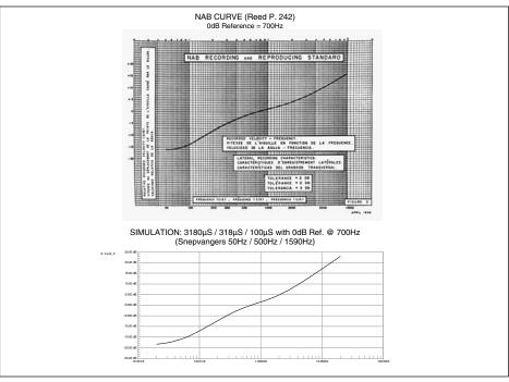
Figure 9. The NAB graph, published by Reed, is shown in the top illustration. NAB put the 0dB reference at 700Hz, rather than at the customary 1kHz, which has caused considerable confusion over the years. The bottom graph is a simulation of the NAB curve using 50Hz, 500Hz and 1590Hz (3180µS, 318µS and 100µS). The 0dB reference in the simulation has also been placed at 700Hz, to allow meaningful comparisons to the NAB graph.
