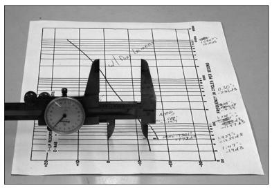
Figure 3. Measuring the Snepvangers graph using precision dial calipers.
