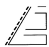
Top bar shows signal strength too high. This will degrade the performance by overloading the input stages. Use an attenuator.
