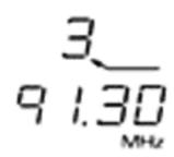
Example: To tune-in Radio 3 (91.30 MHz, Wrotham) and store it into preset position 3:- Press appropriate track <> button until 3 is shown in the display (3 also boxed and arrowed), keep pressing search <> buttons until the station is heard and 91.30 MHz is displayed. Finally press store for about 5 seconds to put the station into the tuner memory.
