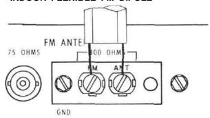
A convenient flexible indoor FM dipole (300 ohm) antenna is supplied with the MR 71 tuner. This antenna is easy to install. It is suitable for a good FM reception in high signal areas.
