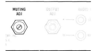
The MR 71 ultrasonic muting circuit suppresses all noise between stations. It suppresses all weaker stations not strong enough to override the background noise.
