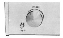
Controls volume level when the tuner is connected to the pair of jacks marked FRONT PANEL CONTROLLED.
