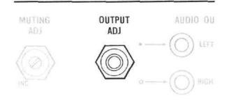
The dual concentric OUTPUT ADJ controls (on the tuner back panel) adjust the output volume level of the left hand pair of AUDIO OUTPUT JACKS. The center shaft of the control adjusts the left channel output. The outer sleeve of the control adjusts the right channel output.
