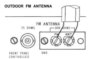
An outdoor FM antenna is recommended for best FM reception under all conditions. In fringe areas, a highly directional FM antenna used with a rotator will give the finest possible FM reception. Rotate the antenna until it points in the direction of the station or until it receives the best possible signal. Use the multipath, signal strength and tuning indicators to position the antenna correctly.
