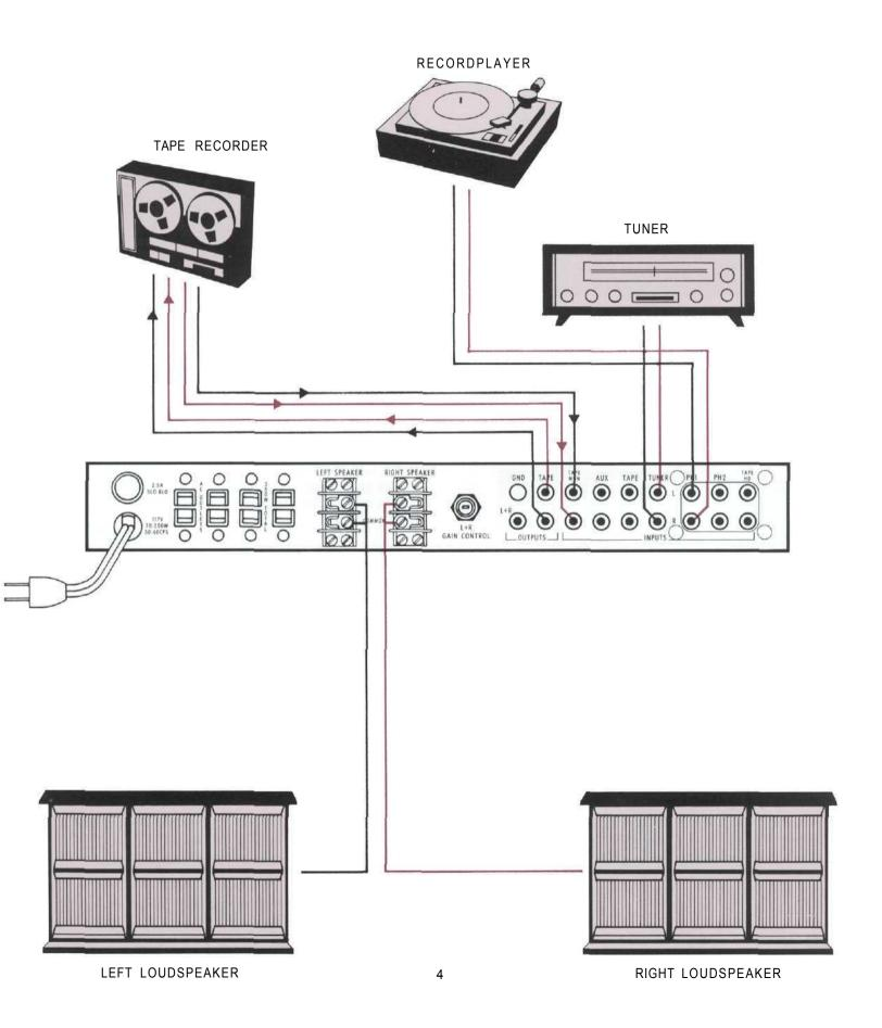
a tape recorder to the L TAPE MONitor input.
