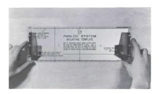
Place the template over the mounting screws. The mounting screws should be centered in the "A" and "B" holes on the template. The sides of the mounting brackets should match the vertical dash lines on the template. If necessary, loosen the screws and push the brackets into alignment and retighten.
