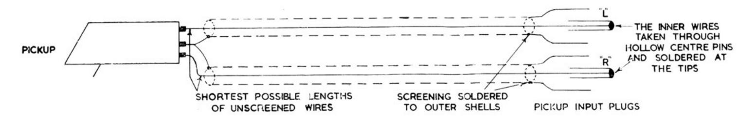
(c) Some pickups will be fitted with two inner conductors covered by one outer screening; in this case the user should make sure that the screening of both inner conductors is maintained right up to the plugs fitting the sockets marked "PICKUP", as shown below.
