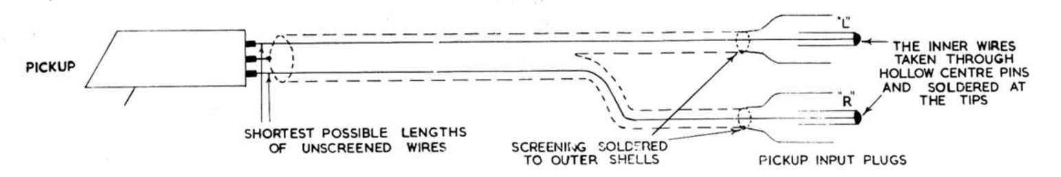
(d) The majority of stereo pickups made today are suitable for reproducing from monaural records when the two outputs are short-circuited; the "FUNCTION" switch on the pre-amplifier effects this short-circuit when turned to "MONAURAL P-U". Some pickups are made which do not conform to this convention; in these cases it will be necessary to use an external switch as supplied or directed by the makers. The diagram below shows a suitable switching arrangement.
