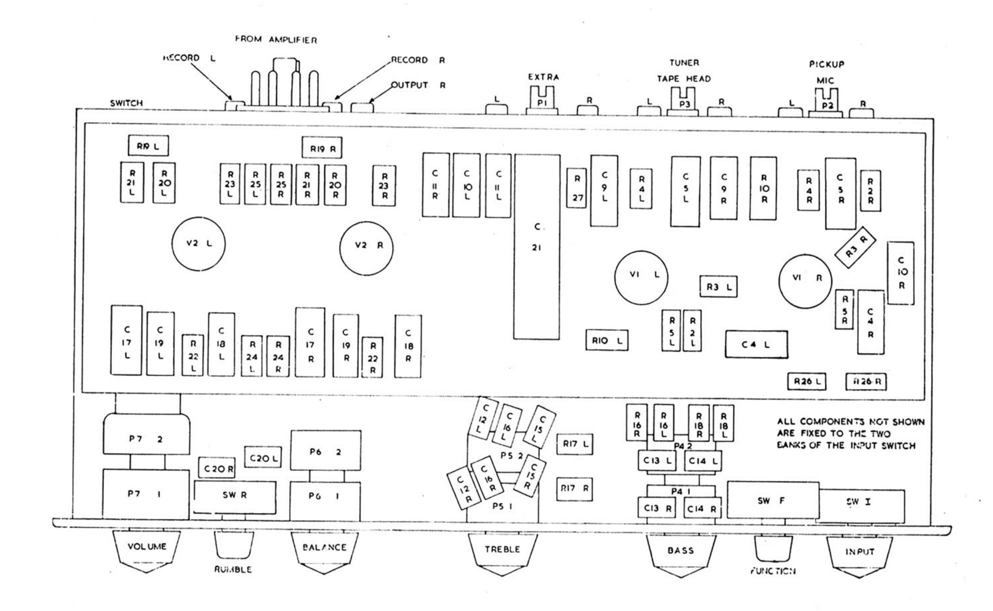
CHASSIS LAYOUT, BOTTOM COVER REMOVED
