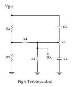
In order to facilitate calculations, we shall first find the Thevenin equivalent for  $V_g$ ,  $R_1$  and  $R_3$ . In fig.7, the equivalent Thevenin voltage source,  $V_1$ , is given by:
