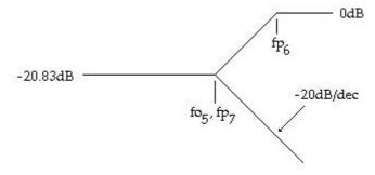
Fig.8 Bode plot of the treble response
