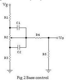
Here,  $R_4$  offers some isolation between this stage and the treble control section (frequencies above the center frequency are affected by this control).  $R_5$  represents the input resistance of the amplifier connected to the output of the James network and should be selected such that it imposes no appreciable load on the network. Here we assume that  $C_3$  and  $C_4$  are open circuits at the bass frequencies.
