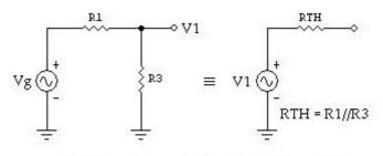
Fig.7 Thevenin equivalent for Vg, R1 and R3
